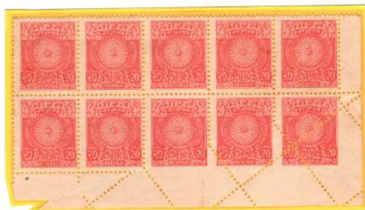
20 (paise) old design south east corner block of 10 with pre perforation paper fold affecting the bottom row resulting in zig zag perforation & impression of partly imperf at places, after straightening the paper fold.
